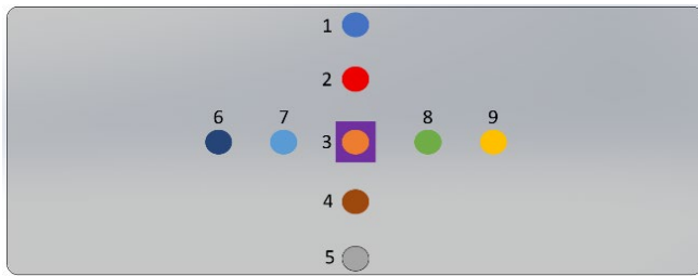
Figure 9: Thermocouple locations on one side of board for full study of hot plate and hot air, where the purple box is the hot air nozzle location. Same set up for both the 13- and 20-layer boards.
