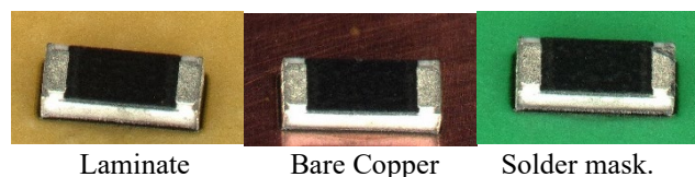
Figure 3. Adhesion test sample assembly schematics and actual component placed on different substrates.
