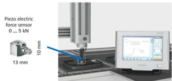
Figure 9: Force measurement w/ evaluation system
