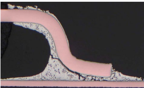
Figure 51: TQFP-144 SAC7.5Bi Solder, Failed at 3123 Cycles
