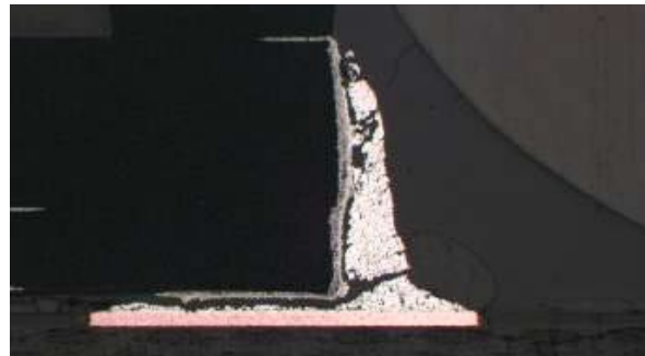
Figure 23: CLCC-20 SnPb Solder, Failed at 328 Cycles
