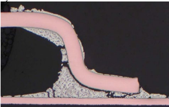
Figure 50: TQFP-144 SAC6.0Bi Solder, Failed at 383 Cycles
