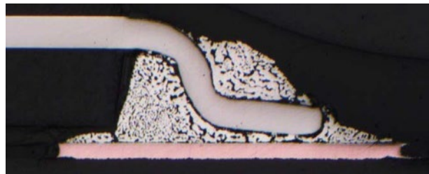
Figure 40: SOT-23 SnPb Solder, Failed at 3004 Cycles
