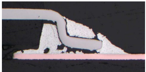
Figure 42: SOT-23 SAC4.8Bi Solder, Failed at 2741 Cycles
