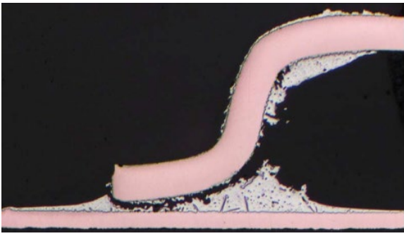
Figure 48: TQFP-144 SAC305 Solder, Failed at 629 Cycles
