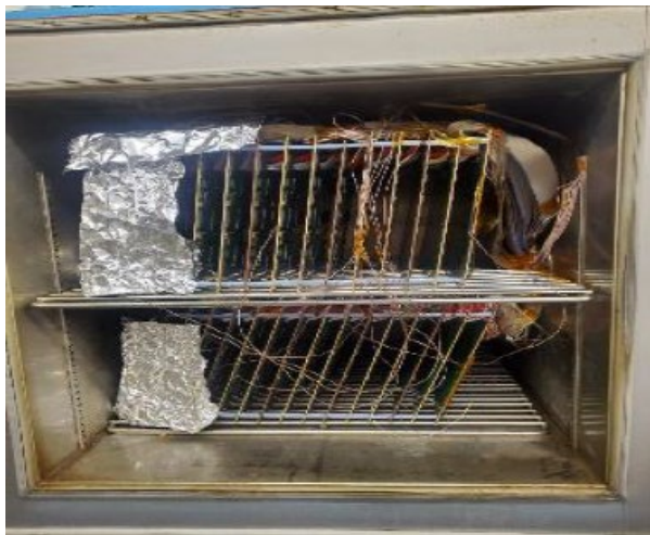
Figure 4: Test vehicles positioned in the thermal cycle chamber
