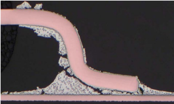
Figure 49: TQFP-144 SAC4.8Bi Solder, Failed at 121 Cycles
