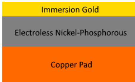
Figure 2. ENIG surface finish, including the problematic nickel-phosphorous (Ni-P) layer. Layers not to scale.
