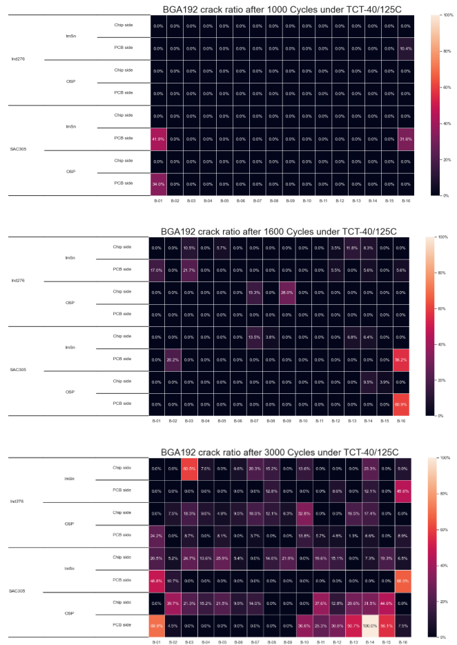
Figure 15. The crack ratio of each joint/ball at both the component side and PCB side in SAC305 and IND276 at 1000, 1600, and 3000 cycles under TCT -40/125°C.
