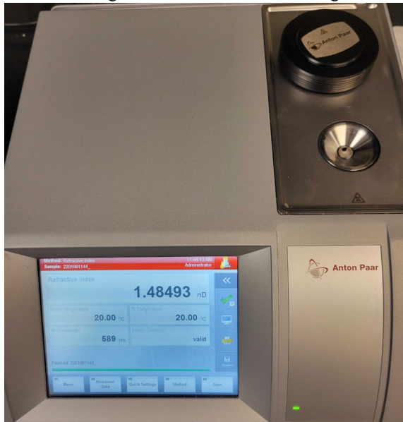
Figure 6. Refractometer used for conformal coating measurements
