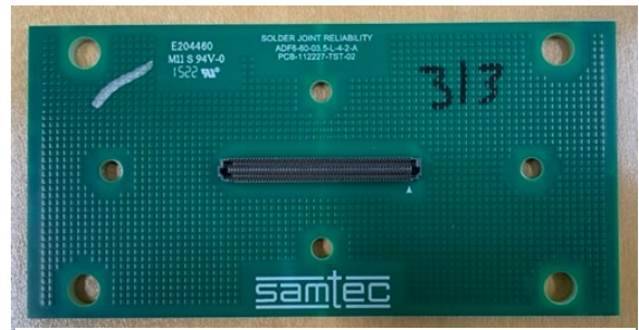
Figure 22. Test Vehicle Layout used for IPC-9701 Testing (Receptacle Side)
