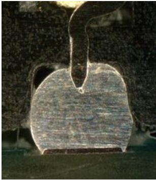
Figure 8. Current Generation Pin-in-Ball Grid Array
