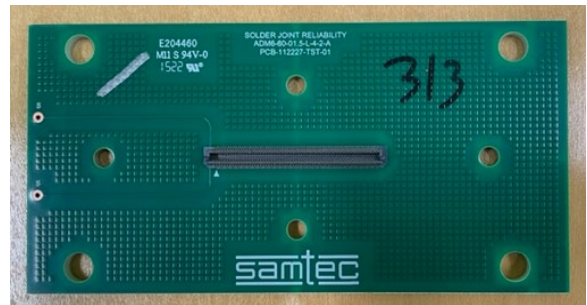
Figure 21. Test Vehicle Layout used for IPC-9701 Testing (Plug Side)
