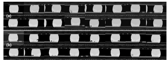
Figure 4. T0 CABGA192 hybrid solder joints of (a) SAC305/Bi+ and (b) SAC305/SnBi1Ag for samples that were thermal cycled at -40/105°C.
