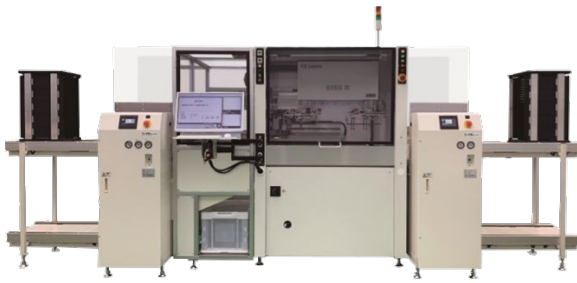
Figure 14: Fully Automated PCB Depaneling Router
