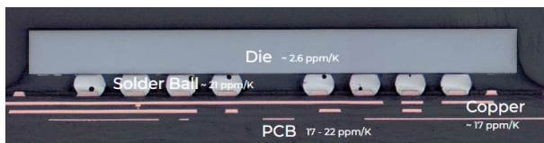
Figure 9. Cross Sectional View of WLCSP
