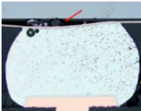
Figure 1. Chip Scale Package Pad Deformation during Reflow Soldering
