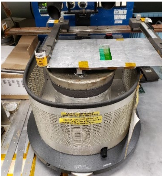
Figure 3: AirVac Mini-wave system with test coupon/soldering fixture
