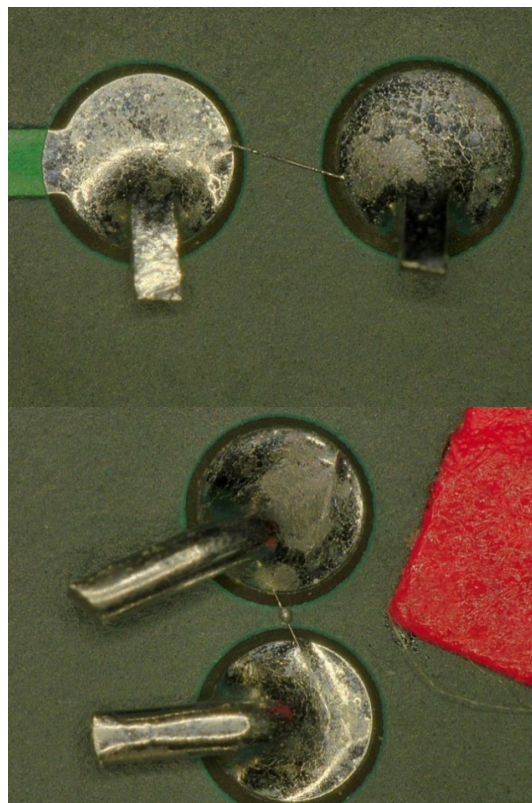
Figure 24: FeSn 2 IMC Phase Shorting Defect
