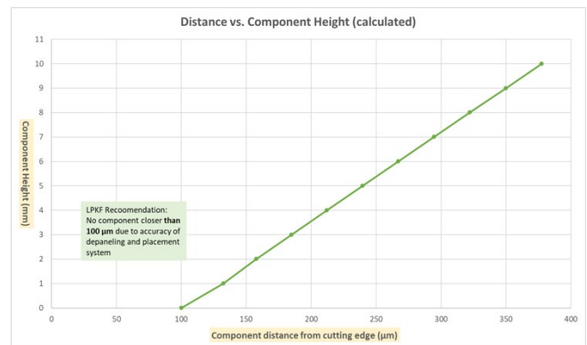
Figure 1. Minimum calculated distance of a component depending on its height for green nano second laser
