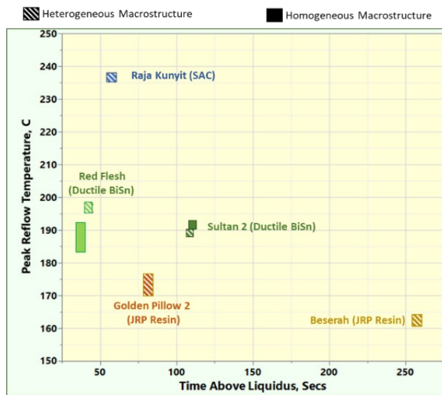
Figure D-1. The Peak Reflow Temperature (C) and Time Above Liquidus (seconds) for the alloys used in this study [37].
