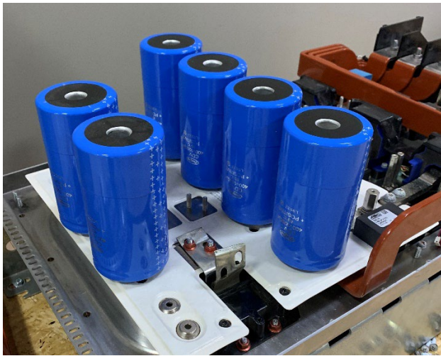
Figure 8. Representative image of drive capacitors
