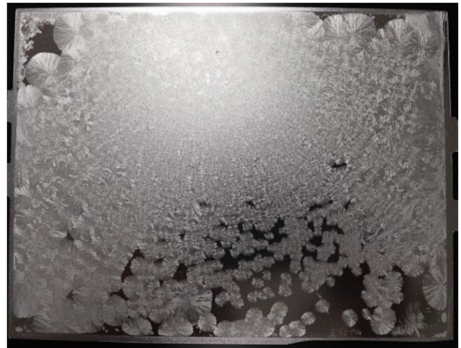
Figure 13. Image of anomaly on diffuser film of returned computer that had been stored with a VCI emitter.
