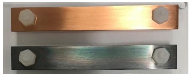
Figure 3. Image of the copper and silver coupons after exposure in the control room. The accelerated silver corrosion is typical of certain types of sulfur contamination in the environment.
