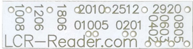
Figure 3. Capacitance offset calibration board.
