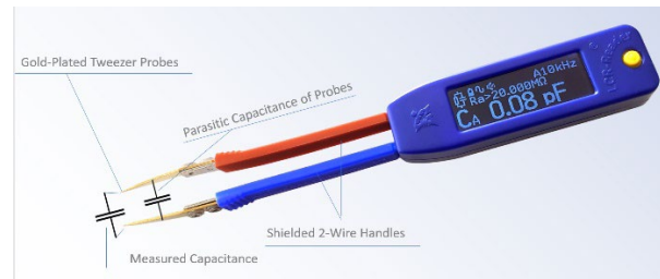
Figure 1. Capacitance offset introduced by test leads of LCR-Reader R2.
