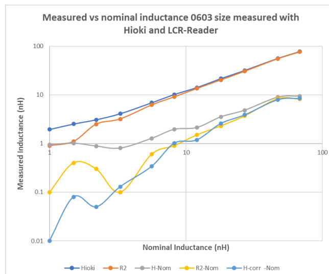
Figure 7. Inductance of 0603 components measured using LCR-Reader R2 with and without short calibration using Short Calibration Board. Compared to measurement results using Hioki IM3536 with and without test fixture offset subtraction.
