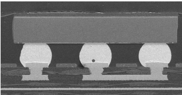
**Figure 14.** Mechanical shock – passed unit.
