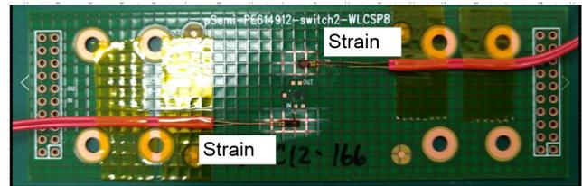
**Figure 8.** Mechanical Shock Test Set Up
