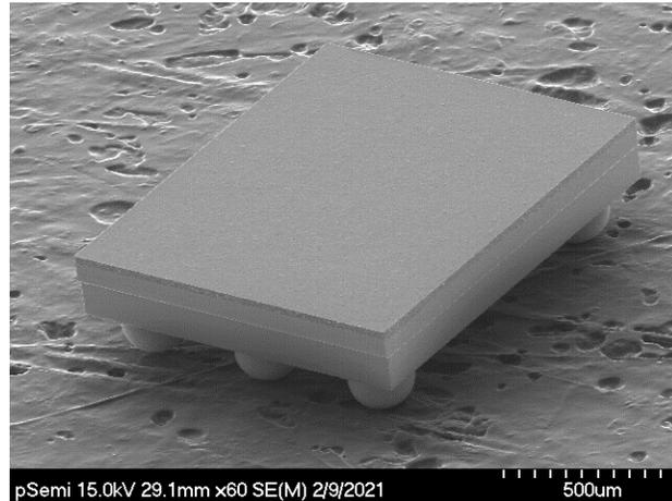
Figure 1. WLCSP Top View
