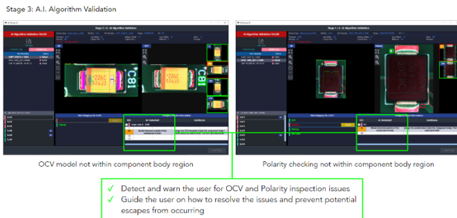
Figure 6. AI Quality Check, Polarity and OCV Defect Simulation
