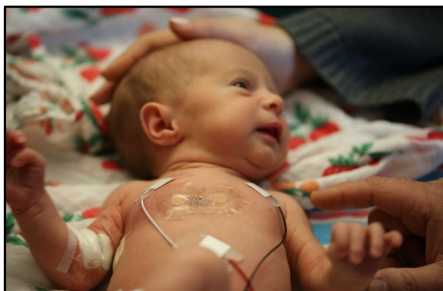
Figure 7. Skin-like devices for wireless monitoring of vital signs in neonatal intensive care [24].
