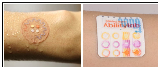
Figure 9. Skin-like microfluidic systems for real-time analysis of sweat [24] [26].
