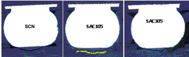
Figure 13. Pad cratering was seen on all samples.
