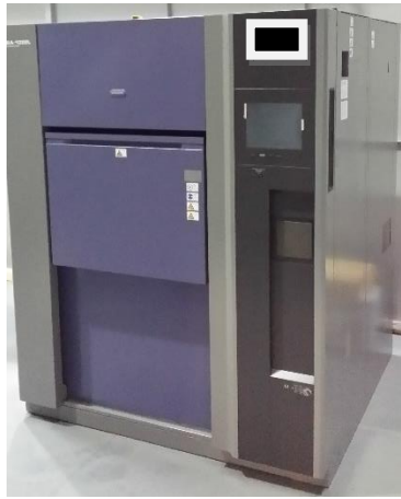
Fig 9. Production thermal shock chamber
