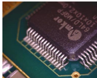
Fig 4. QFP leads at alternating polarity.
